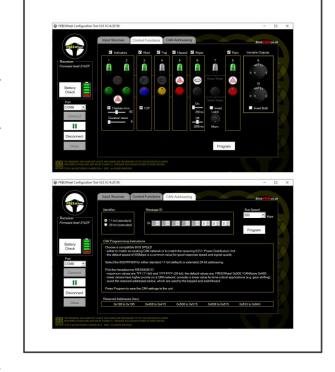
Pressing steering wheel buttons connected to the Transmitter will illuminate the corresponding buttons and toggle or flash the virtual relay states on the software.
