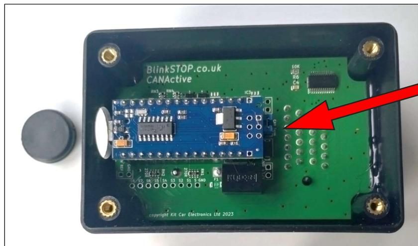
To access the USB port, carefully prise off the grommet using a small screwdriver and refit after use.
